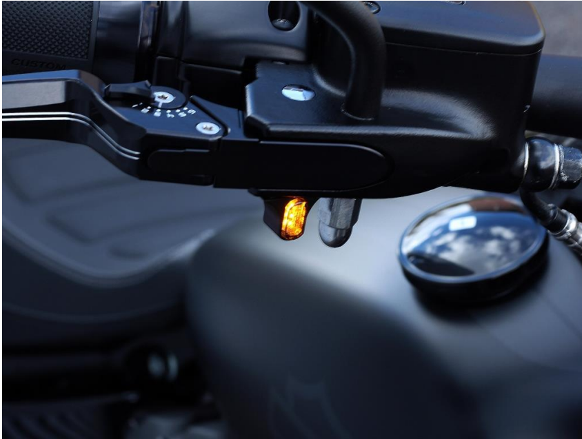
Picture 2 of 3: Simple and clever: Turn signal for gluing
