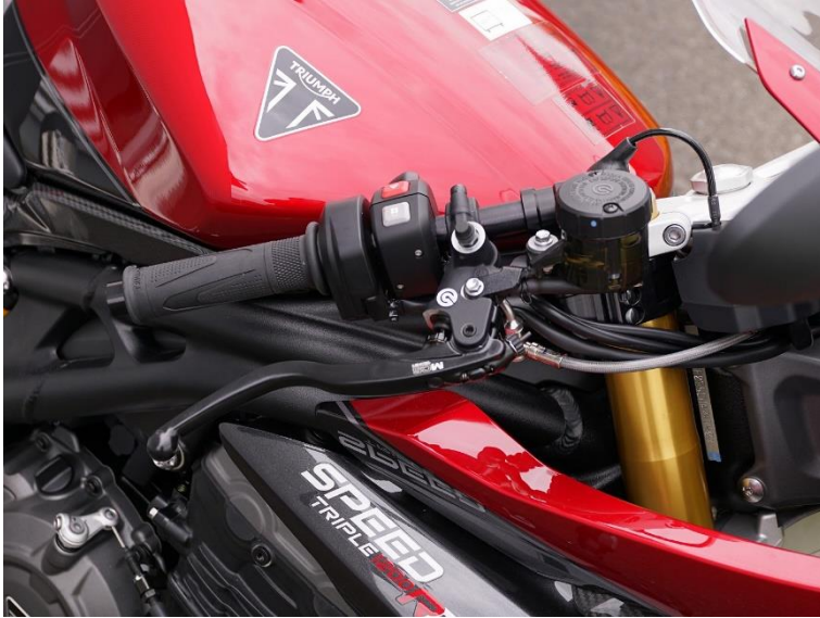
Pic 4: Complete clip-on conversion in a ready-to-install mounting kit
