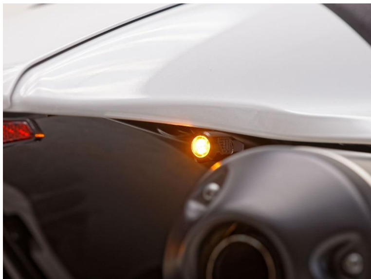
LED indicator/taillight combination for rear mudguard
