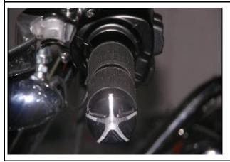
Slide the new grip onto the handlebar and fasten the grub screws provided.
