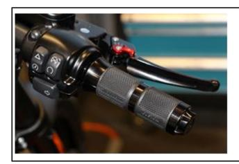
When the axial backlash is too big, clip the provided plastic washer into the guide between grip and switch housing.
