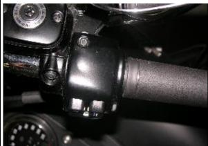
Loosen the upper screw and remove the lid.
