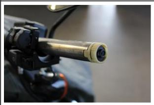
Pull the throttle grip sleeve from the lever.
