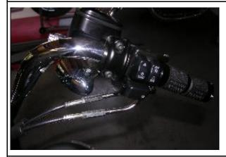
Lightly pull down the protective rubber of the cables and remove their counter nuts.
