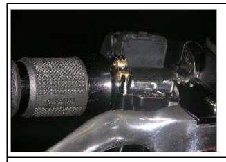
When the backlash is too big, clip the provided plastic washer into the guide between grip and switch housing.
