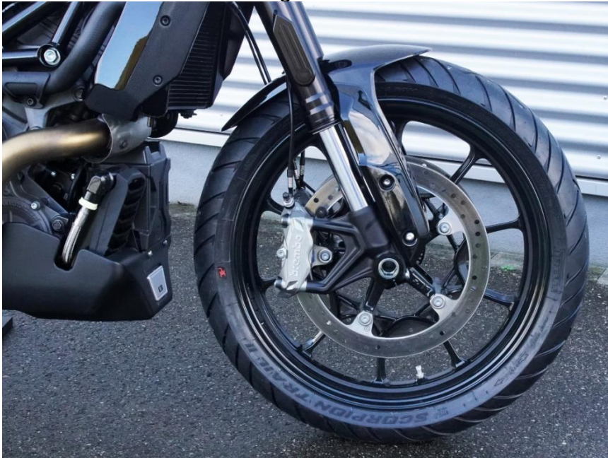
Pic 12 of 13: Set for lowering the front fender
