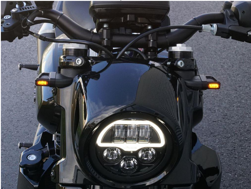
Pic 6 of 13: Also for the front, new LED indicators
