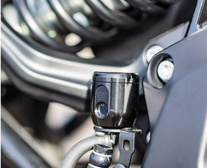
Pic 11 of 13: Fluid reservoir for foot brake & handbrake fitting
