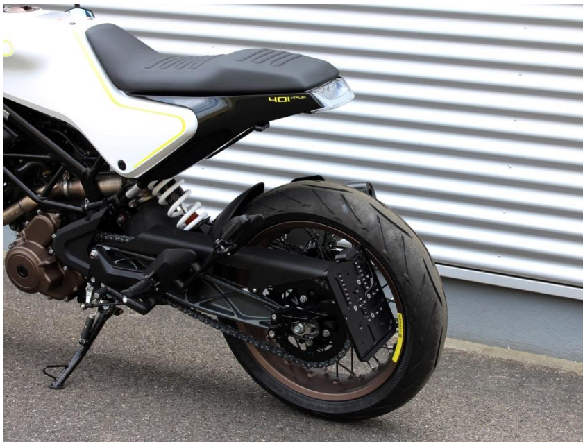
Side mountable licence plate holder Husquvarna Vipilen 401
