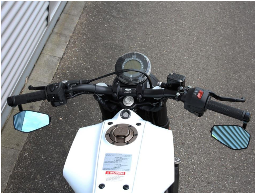
Superbike handlebar conversion with „booster“ handlebar Husquvarna Vitpilen 401
