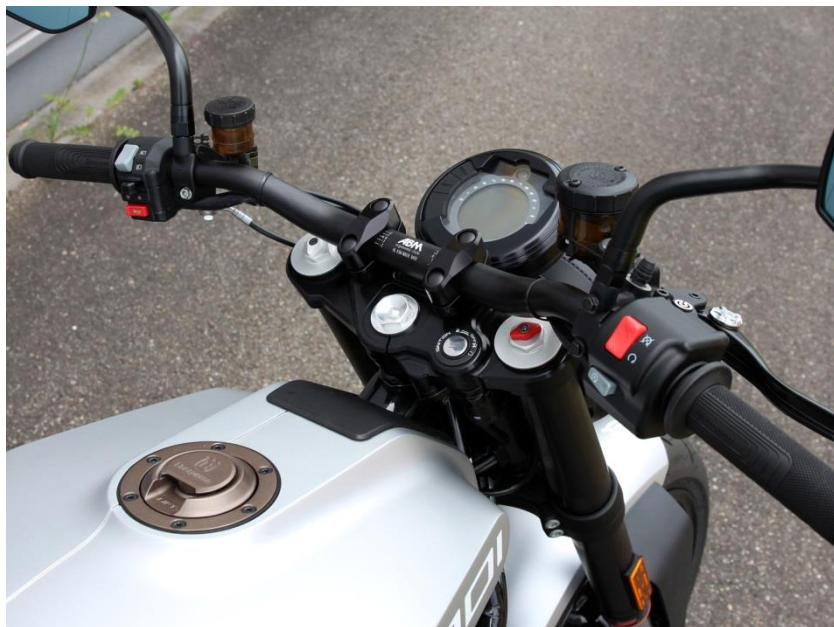
Superbike handlebar conversion with „booster” Husqvarna Vipilen 701
