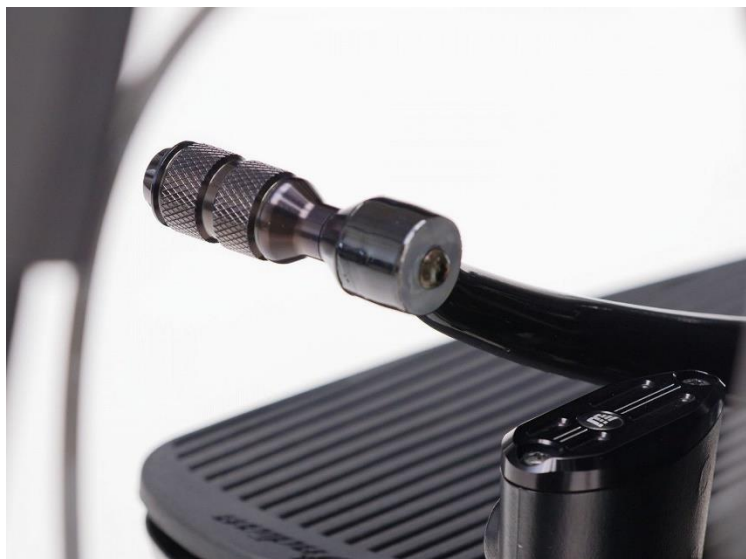
Replacement pedal for the foot brake lever
