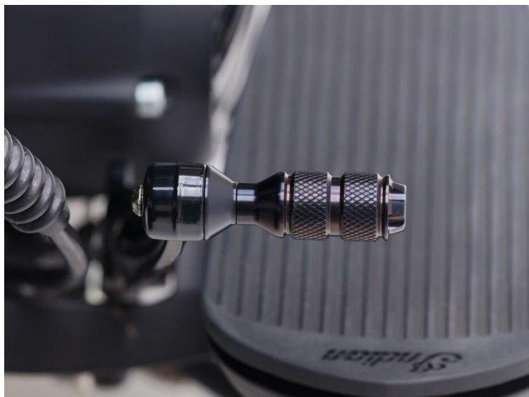
Replacement pedal for the gearshift lever
