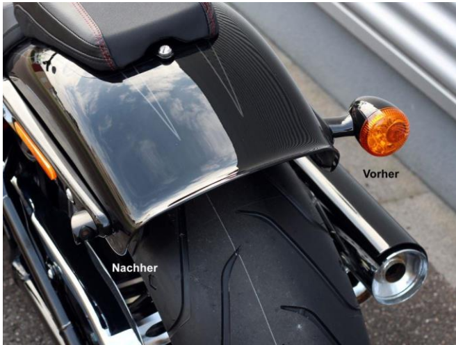
Picture 5 of 5: Before – After: Replaces the stuck out original light units
