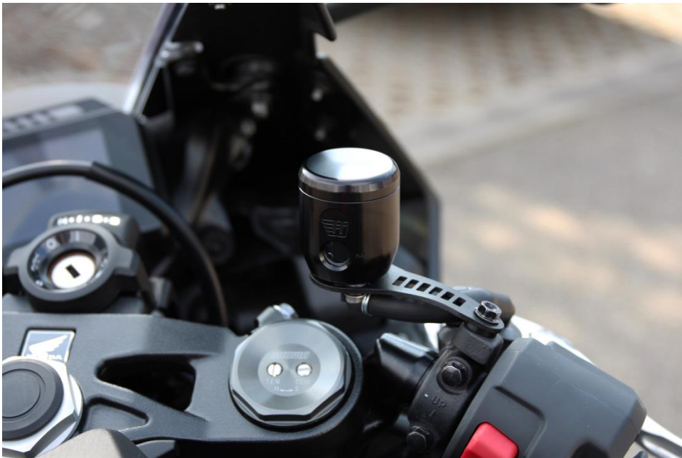
Pic 2 of 4: 90° bracket which is rotatable by 360°
