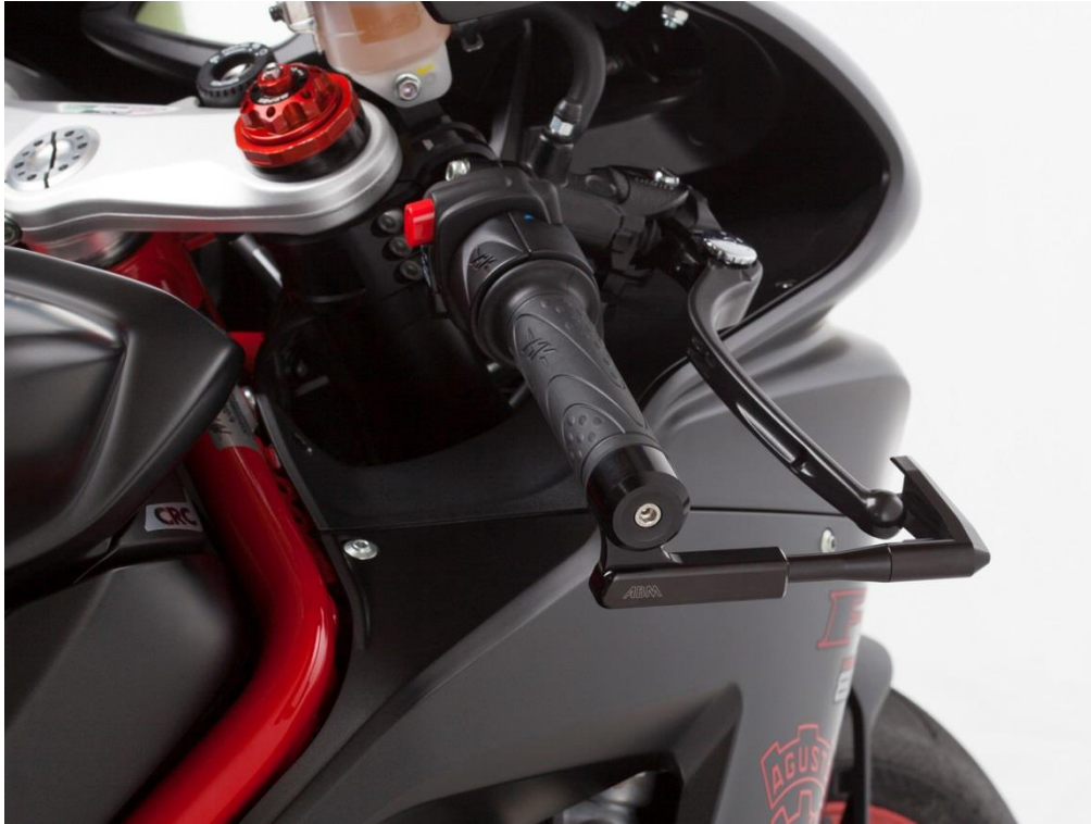
Pic 4 of 4: leverSafe protects against contact with other riders or obstacles
