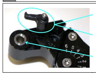
KH39: Requirement for S1000**R and** S1000**RR**: The actuating part for the clutch switch of the original lever must be mounted.
