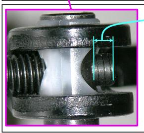
Precisely measure the shown distance with a sliding calliper and record this measurement.
