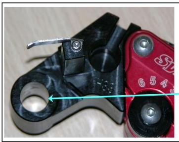
Requirement for S1000RR until 2014: The original guide bushing must be used.
