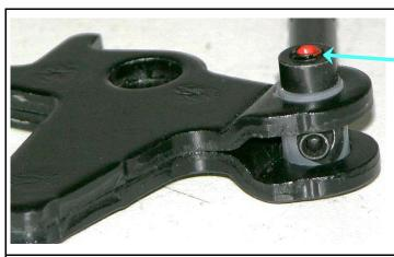
Heat the grub bolt sufficiently with a hot air gun to unblock thread-locker and demount it.
