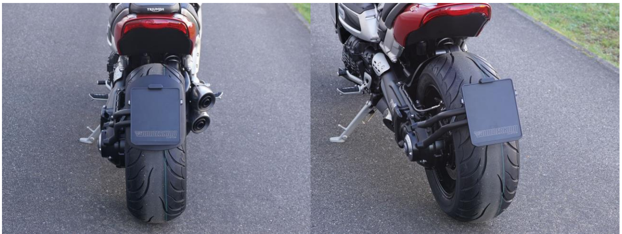
Central license plate holder with or without original splash guard
