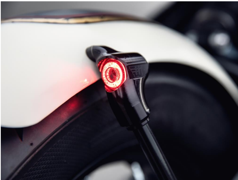
Picture 2 of 4: Struts with integrated turn signal, rear & brake light
