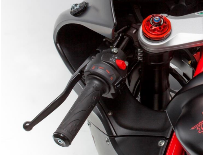
Picture 4: Adjustable clip on bar 'raceClip' for racing - tested & certified!
