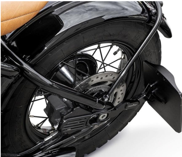
Installed TWINTON® license plate holder - side mount
