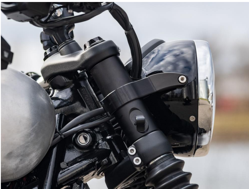
Installed TWINTON ® lamp arm
